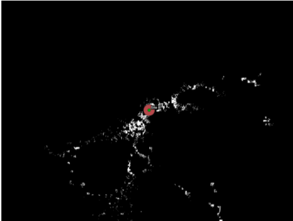
The white areas show terrain with greater than 50% mean illumination and less than 5° mean slope within Shackleton-de-Gerlache Ridge. Site B is the chosen location. The surrounding red circle shows the 200m buffer.
