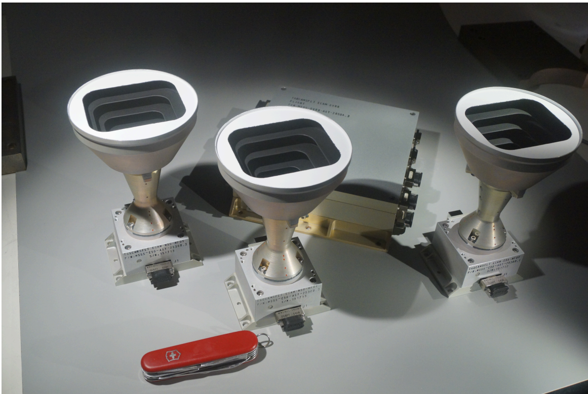
Figure 2.1.5.2.1: TAGCAMS DVR and Camera Configuration
